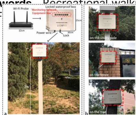
The demonstration of the integrated Wi-Fi device box (a) and its installation (b)
